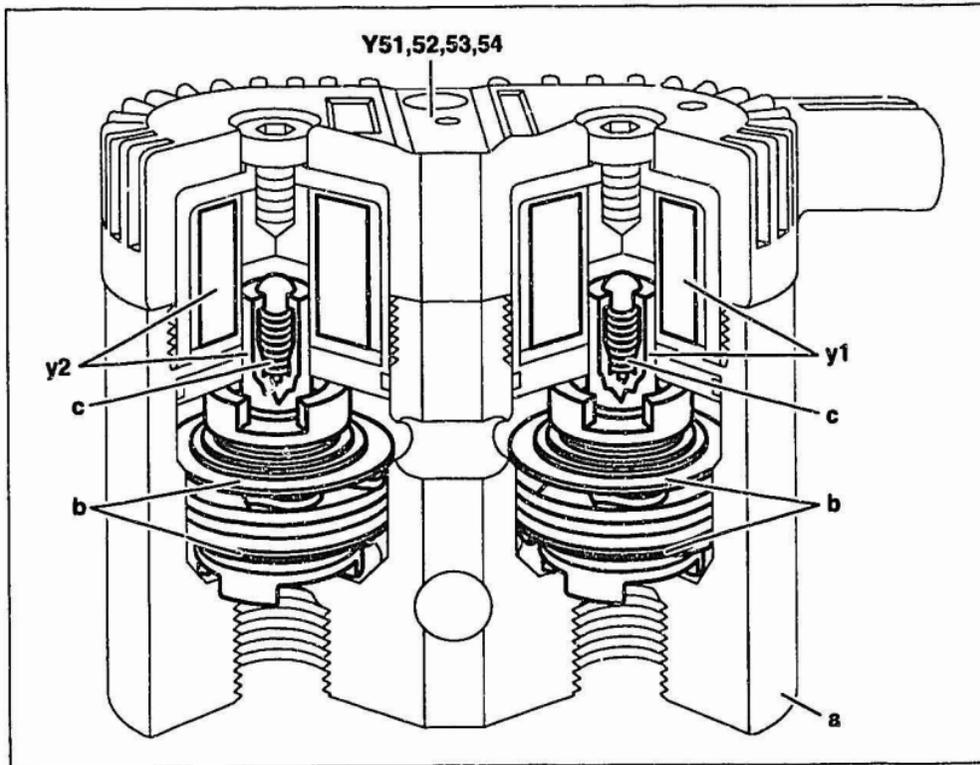
The damper valve (Y51, Y52, Y53, Y54) consists of the housing (a) and the 2-piston/reed valve packages (b). The spring-loaded (c) solenoid valve pistons and the solenoids in the upper section of the housing are located above these. The valve pistons and solenoids form the solenoid valve units (y1, y2).
