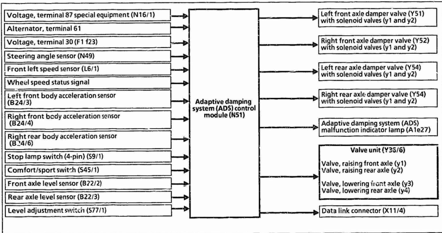
The corresponding functions of the hydraulic control circuit are controlled with the electrical/electronic components.
